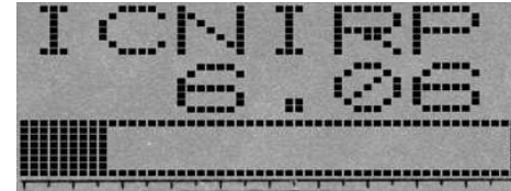
SPECTRAN® displays exposure limits both as percentage as well as a bargraph display.
