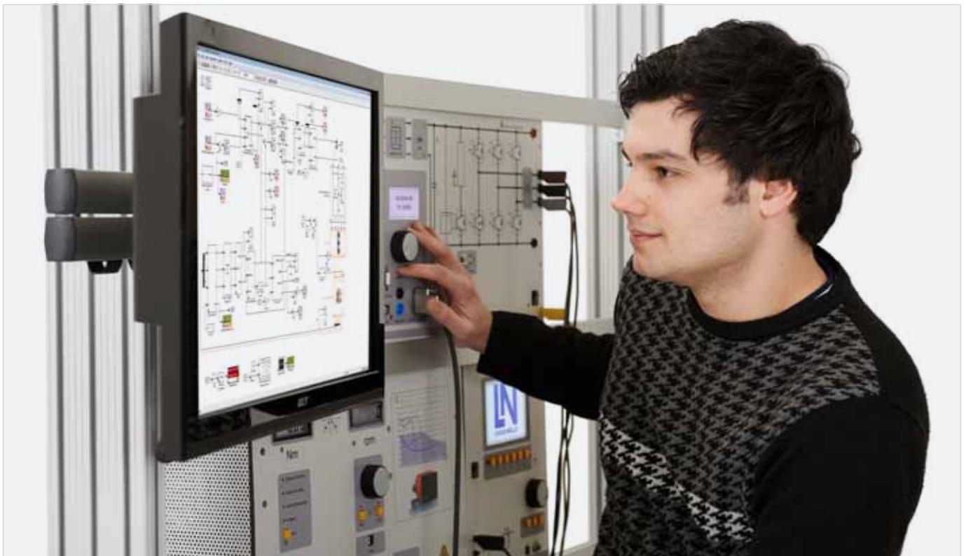
Training system: "Field-oriented control of asynchronous motors with Matlab®/Simulink®"
