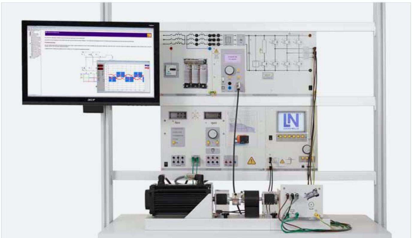
Training system: "Servo-drives with a servo-machine test stand"
